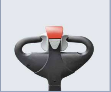
The unique creep speed driving function allows the truck can be driven slow easily, and more accurately.
